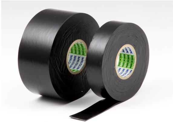
Nitto 15 is a self fusing rubber tape, widely used for electrical insulation, protection, splicing and termination of 6 to 22KV cables.
