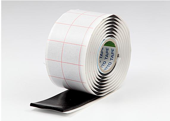
Nitto 12FB is a self amalgamating putty tape. By stretching and wrapping around pipefittings, cables, or other objects, the putty will instantly amalgamate into itself, thus creating a waterproof barrier to prevent corrosion. 12 FB is suitable for in and outdoors.
