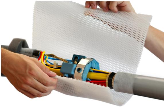
A 3D Gauze is used in the construction FiloSlim injection joints. Two layers of the 3D gauze create the correct insulation space for conductive parts in the joint. The joint's high elasticity gives the joint an elegant and smooth shape. The FiloSlim 3D gauze sheet's open structure enables an even distribution and flow of resin in the FiloSlim injection joint.
