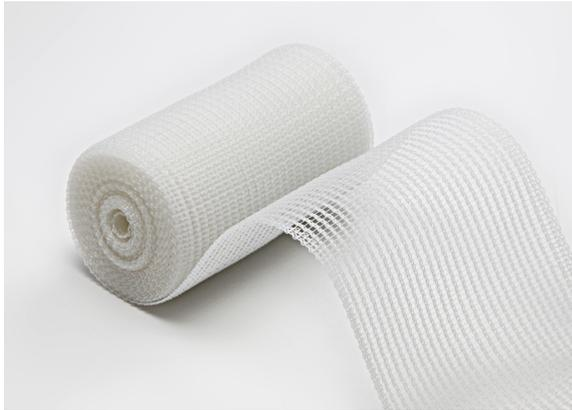
Flexible gauze is used to create insulation distance around the conducting parts when making an injection joint. It also contributes to an optimal distribution of the resin in the injection joint. Because of the width, the 10 cm wide version is very suitable for the insulation of the earth screen as well as for wrapping up the total joint.
