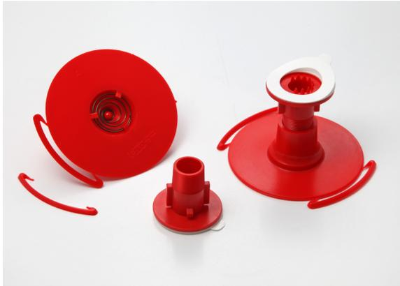
Filoform injection nozzle and injection valves are used for injection joints. The injection valve is positioned on the wrap around gauze by using the wrap around tape. The injection nozzle is placed onto the resin pack in order to enable an easy and smooth injection of the resin into the joint. Recommended for injection joints on cables  $>4 \times 25\text{mm}^2$
