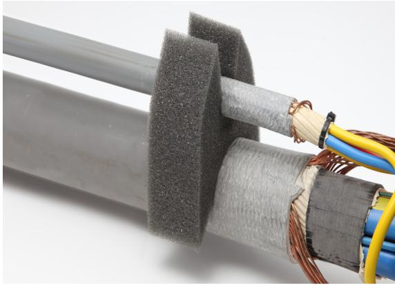
The Filoform Branch seal is used in taped resin joints with branch configurations. The branch seal is a polyether molded product, which seals the space between the main cable and the branch cable, allowing de-airation of the joint. The innovative design ensures efficiency combined with minimal material wastage.
