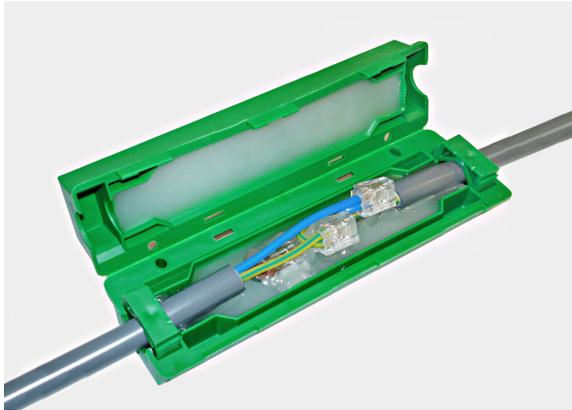
The smart Joint is a cable joint which is pre-filled with an insulating and waterproof filling mass, and is suitable for cable diameters up to 15.7mm (0.62 inch); 2 x 2.5mm<sup>2</sup>. The Smart Joint can be used inside and outside as well as underground
