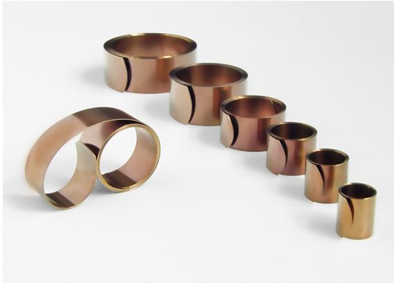
Constant force springs are the ideal method to complete electrical continuity across the joint on armoured power cables for straight or branch joints. Using constant force springs is an easy and reliable way to earth the cable joint as they constantly exert pressure on the earth braid to achieve a reliable continuity.
