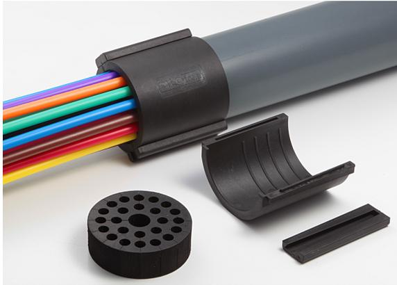
Suitable for Gas and Watertight sealing of 63mm HDPE ducts, which contain mini/micro ducts and / or (fibre optic) cables. The modular system will guarantee easy installation of various different cable and duct configurations. Our system is divisible so can be applied at installation or afterwards. The rubber inserts can be custom designed for your specific needs and configuration and will contain (temporary) blind plugs to make the system more flexible at the installation site.
