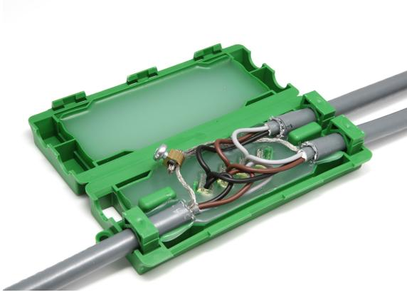
The smart Joint is a cable joint which is pre-filled with an insulating and waterproof filling mass, and is suitable for cable diameters up to 15.7mm (0.62 inch); 4 x 2.5mm<sup>2</sup>. The Smart Joint can be used inside and outside as well as underground
