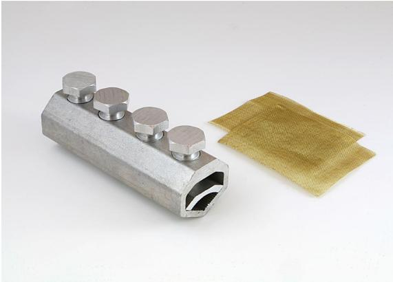
Joining of stranded aliminum or copper cores in appliactions up to 11KV Shear off screws to ensure a consistant and reliable connection Supplied with brass gauze to improve electrical stability when joining copper cores.
