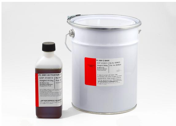
Filoform's Slot cutting resin PC5581D is a cold curing 2 component polyurethane resin specially designed for backfilling of cut slots for detector loops on motorways and all purpose trunk roads. PC5581D has good adhesion and meets all specifications as set by the Highways Agency for encapsulants.
