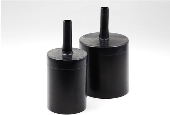
Heat Shrink Anode Caps are used to seal and protect the critical connection between the lead wire and anode. It provides stress relief, moisture proofing and electrical insulation at the lead wire exit point. It is an ideal solution to the problem of premature system failure due to corrosion causing the lead wire to come out of the anode.
