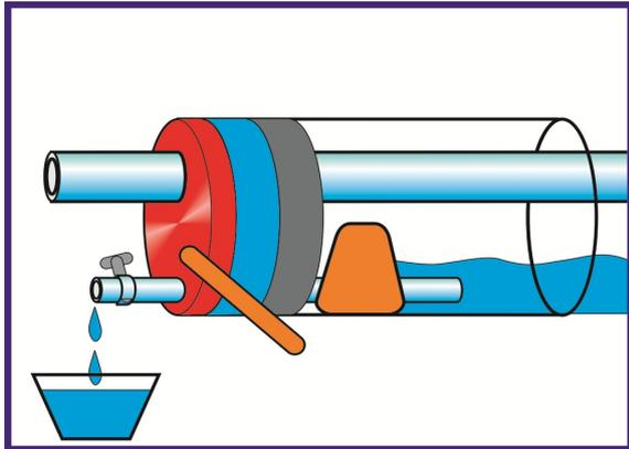
One of the reasons why ducts are sealed is to prevent running water getting into a building or enclosure. Often when faced with sealing a duct, this running water is still evident. Our Filoseal Running Water Block system provides the user with a method of preventing the water from ruining any permanent sealing system whilst that system is installed. The kit provides a method of damming the water flow, controlling it and stopping it.
