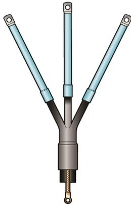
6/10(12)kv - Three core Filoform Medium Voltage Heatshrink Termination Kits are tested in accordance with CENELEC 629.1.S2 & IEC 60502-4, and suitable for Indoor applications up to 6/10(12)kv.
