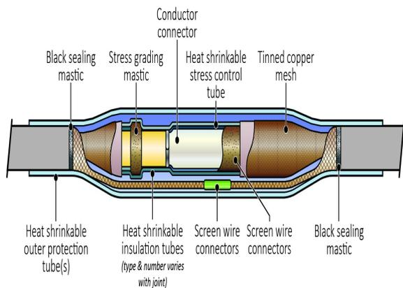
6/10(12)kV - Single Core - Filoform Medium Voltage Heatshrink Straight Cable Joints, are manufactured and tested in accordance with CENELEC 629.1.S2 & IEC 60502-4, and suitable for Indoor and Outdoor applications for 6/10(12)kV.
