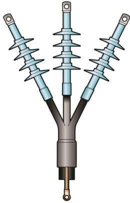
6/10(12)kv - Three core Filoform Medium Voltage Heatshrink Termination Kits are tested in accordance with CENELEC 629.1.S2 & IEC 60502-4, and suitable for Outdoor applications up to 6/10(12)kv.
