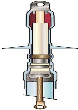
6/10(12)kV - Single core Filoform Medium Voltage Heatshrink Termination Kits are tested in accordance with CENELEC 629.1.S2 & IEC 60502-4, and suitable for Outdoor applications up to 6/10(12)kV.
