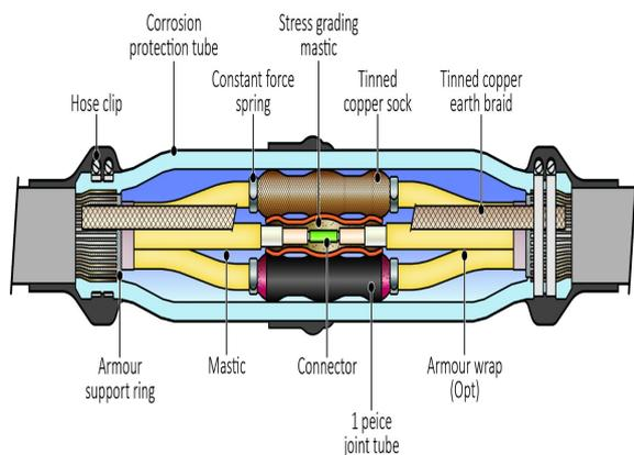
8.7/15(17.5)kV - Three Core - Filoform Medium Voltage Heatshrink Straight Cable Joints, are manufactured and tested in accordance with CENELEC 629.1.S2 & IEC 60502-4, and suitable for Indoor and Outdoor applications for 8.7/15(17.5)kV.
