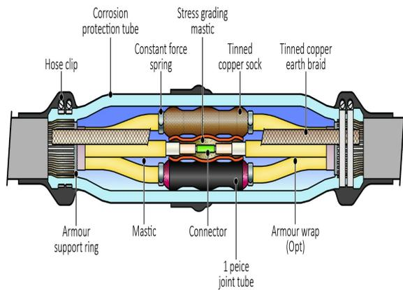
12/20(24)kV - Three Core - Filoform Medium Voltage Heatshrink Straight Cable Joints, are manufactured and tested in accordance with CENELEC 629.1.S2 & IEC 60502-4, and suitable for Indoor and Outdoor applications for 12/20(24)kV.
