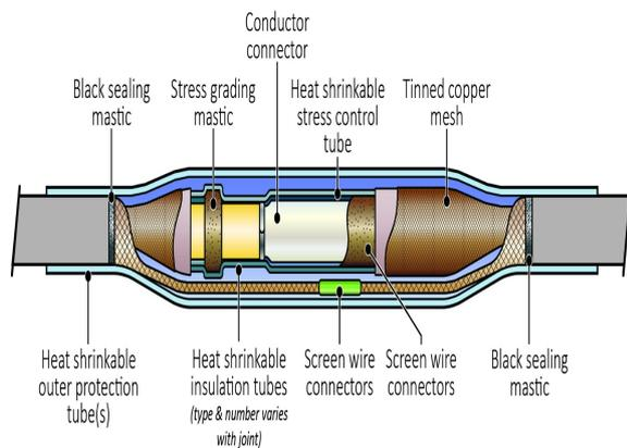
12/20(24)kV - Single Core - Filoform Medium Voltage Heatshrink Straight Cable Joints, are manufactured and tested in accordance with CENELEC 629.1.S2 & IEC 60502-4, and suitable for Indoor and Outdoor applications for 12/20(24)kV.
