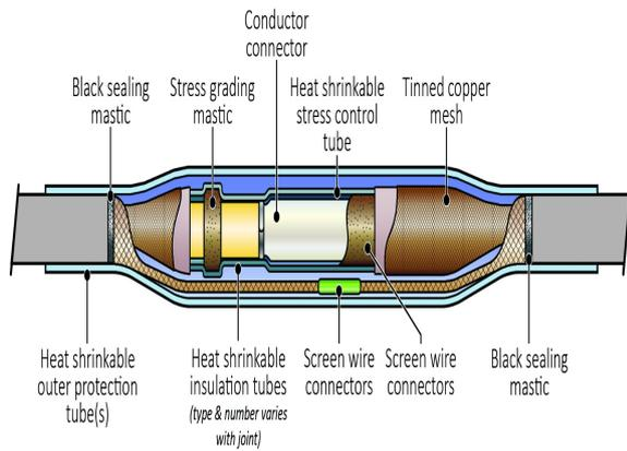
18/30(36)kV - Single Core - Filoform Medium Voltage Heatshrink Straight Cable Joints, are manufactured and tested in accordance with CENELEC 629.1.S2 & IEC 60502-4, and suitable for Indoor and Outdoor applications for 18/30(36)kV.
